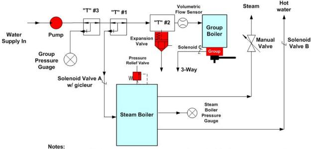
1) The pump does not block water flow when it is not running. When the pump is off, street water pressure remains at the pump outlet in the V2. This means that water pressure is constantly applied through 3-way T #1, through 3-Way T #2, and into the group boiler.
