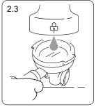
Backflushing. Insert the blind filter (C) into the portafilter and pour 1 bag of detergent powder (F or PLA9201) into the filter. Insert the portafilter (G) in the group (13) and lift the lever (14) for 10 seconds. Stop the function and wait for 10 seconds. Repeat the procedure 10 times (Pic 2.2).
